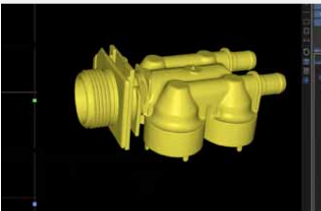
Plastic molded components: dimensional and porosity analysis for production validation.
