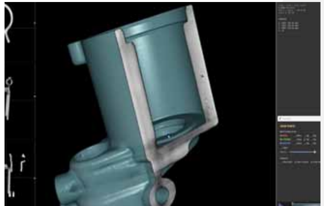
Aluminum die castings: porosity inspection during production start-up.
