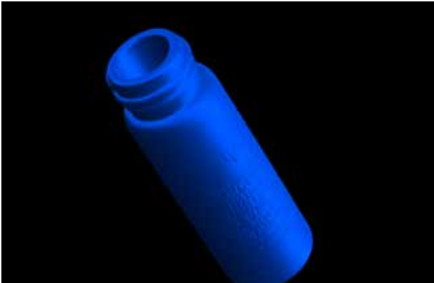
Glass vials: internal dimensions and volume measurement without the aberrations typical of optical measurement.
