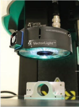
VectorLight™ programmable oblique illuminator highlights surface details from every angle.
