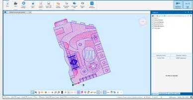
The CMM-like Sampler converts dense and noisy scan data to reliable, sparse, 'CMM-like' point data for standard based dimensional and GD&T evaluation. This tool is feature and CAD model based, and samples points using the CAD model's geometry information.
